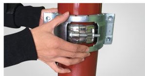
1、將 DS 爪箍的兩半部分均勻地固定在管子的末端，必須確保螺絲和齒型接位於管道上。Fix the two half parts of the DS grip collar uniformly and closely to the end of the pipes, must ensure the collar bolts and teeth are directly located onto the pipe.
